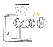
Unlock and twist off the pulp extractor: Grip the pulp extractor and rotate it clockwise to unlock from the juicing chute Carefully move it away from the juicing chute and set it aside. 4.
