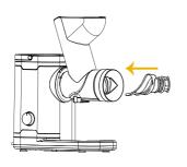
Fit the juice strainer over the auger with the mesh facing downward. The wider end of the strainer should rest underneath the auger. Push towards the motor base until it sits securely in place.
