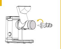
Insert the auger through the centre of the juicing chute and down into the motor base
