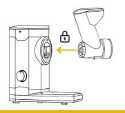
Attach the juicing chute to the motor base Position the chute so it fits into place and moves slightly back into the base. Then rotate it anticlockwise until it locks firmly into position.
