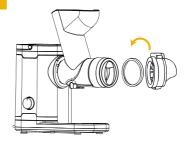
Attach the pulp extractor with the pulp extractor seal to the juicing chute. Align it with the auger, juice strainer and feeding chute, then rotate it anticlockwise to lock it in place. If not installed correctly, there may be a gap between juicing chute and pulp extractor, or the extractor may fall off.
