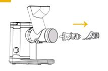
Remove the juicing strainer and auger: Pull out the juicing strainer by removing it from the juicing chute. Then pull the auger out of the chute.
