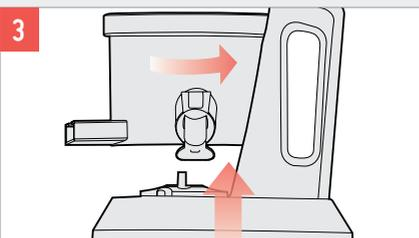
Remove the base. Separate the juicing bowl from the juicer base. Wipe down the base with a damp cloth if required.
