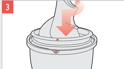
Insert the juicing screw into the strainer. Push it down firmly, and turn it until you hear a click as it locks into place.
