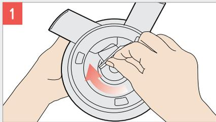
Place the compression silicone piece partway into the slot beneath the pulp spout. Ensure that most (around 60%) of the silicone remains outside of the slot.
