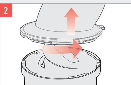
Open the drum lid. Turn the lid anti-clockwise to open it, until the red dot on the lid aligns with the red dot on the bowl again. If the lid is stuck, please refer to the troubleshooting section.
