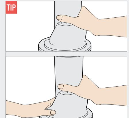
To close the lid, hold the feeding tube in one hand and the bowl in the other; then turn the lid clockwise until the "CLOSE" mark lines up with the red dot on the bowl.
