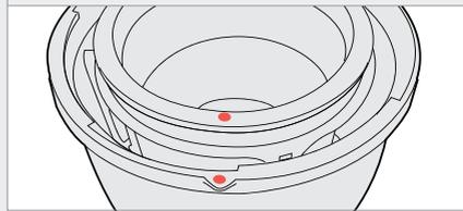
Place the filter inside the silicon wiper unit, then add the wiper unit into the juicing bowl. Line up the red dot on the strainer exactly with the equivalent red dot on the bowl.
