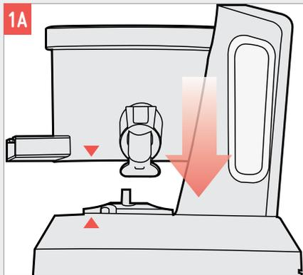
Position the juicing bowl on top of the juicer base. Line the black arrows on the base up exactly with the grey arrows on the bowl.
