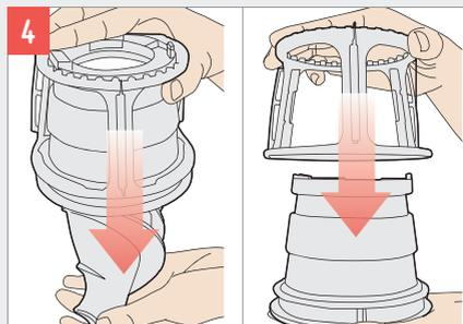
Separate out and clean the juicing components. Remove the silicon wiper unit, strainer and juicing screw from the juicing bowl. Clean them in hot, soapy water using the special juicer brush provided.
