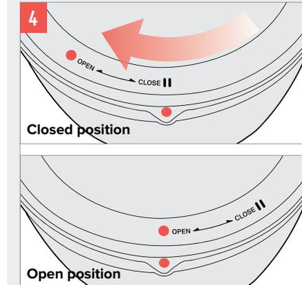
Position the drum lid on top of the juicing bowl. Line the red dot on the bowl up with the equivalent dot on the lid.
